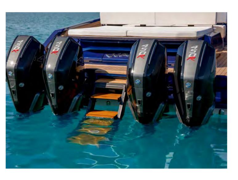
Wally has ingeniously split the four engines to the flanks of the boat, with two on each side, allowing the installation of the retractable hydraulic boarding passerelle/swim ladder to provide direct and easy access to the water or the shore.
